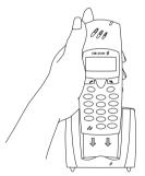
The charging process will start automatically, indicated by a fast flashing battery icon and a green light on the charger. When charging is complete, the icon stops flashing and the green light is turned off.
