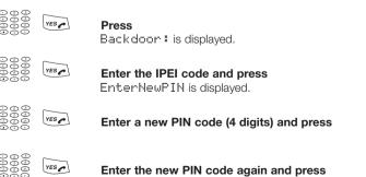
New PIN accepted is displayed for two seconds. The PIN code is changed.
