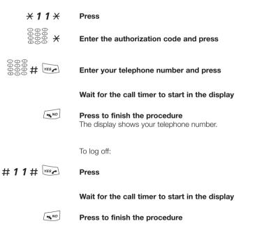
Note: An earlier version of the free seating function use other procedures: To log on, press **X 1 0 X** extension No. **#**. To log off, press **# 1 0 #**.
