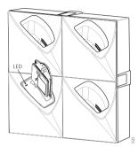
Each power supply module can support three charging racks with four positions for phones in each rack (see technical specifications for the charging rack).
