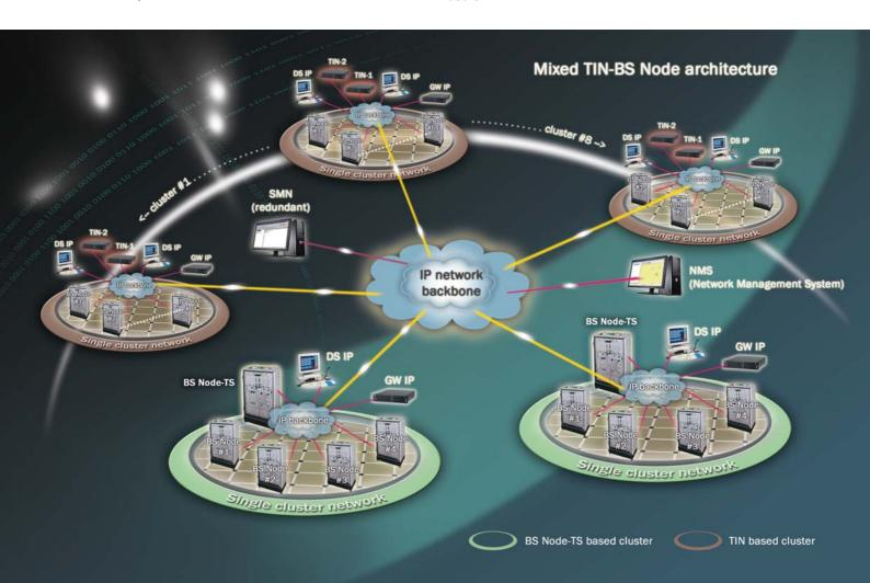
TIN hosts a high speed VLR database and interacts with the SMN to refer to the HLR database to manage the registration of the subscriber positions throughout the network, in order to give to the system the possibility to localise them when called.
